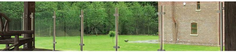
The bolt-down round pre-assembled post system without handrail is designed to cut installation time. It is available in 42.4 & 48mm satin finish stainless steel 304 for internal or 3016 external applications and to suit 10mm toughened glass panels (6, 8 & 12mm rubbers are available to buy separately).
